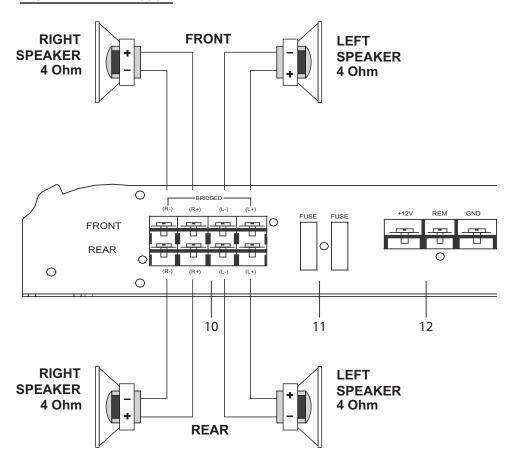
For bridging front and rear into single speaker loads, the XA-6004 has the ability to be bridged as shown in the diagram below:
